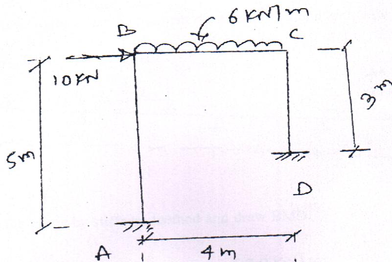
3. Analyse the frame as shown in fig by slope deflection method and draw BMD.
