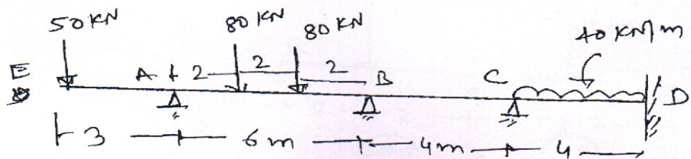
5. Analyse the frame by stiffness method and draw BMD.
