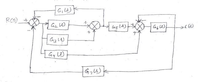
4. (a) Use Mason's gain formula and find the transfer function T(s) = C(s) / R(s) for 10 the system.
