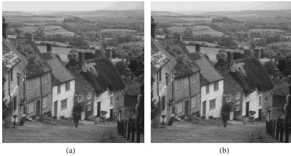
Figure 43: Reconstructed “Goldhill” image: (a) after direct quantization of the original pixels and (b) after quantization of the wavelet coefficients.
