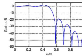
**Example E10.6:** Determine the weighting function  $W(\omega)$  that is to be used to design a Type 1 linear-phase FIR lowpass filter using the Parks-McClellan method to meet the following specifications:  $\omega_p = 0.36\pi$ ,  $\omega_s = 0.58\pi$ ,  $\alpha_p = 0.5$  dB, and  $\alpha_s = 55$  dB.
