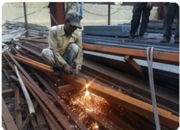
Figure 10 Cutting into billets or blooms using gas cutting
