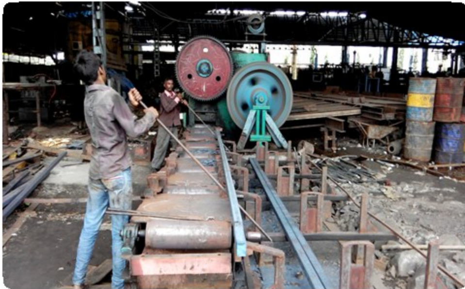
Figure 21 Workers manually lifting the product
