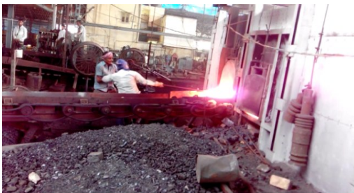
Figure 19 Billet Ejection from furnace
