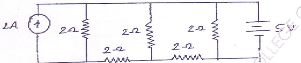
4. (a) In the network shown in figure at  $t=0$ , switch is opened. Calculate  $v$ ,  $dv/dt$ ,  $d^2v/dt^2$  at  $t = 0^+$  10
