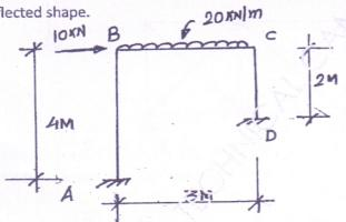
Q. No. 4 Analysis the rigid jointed plane frame as shown in figure, using Flexibility Method .Draw BMD ,SFD and deflected shape. (20)
