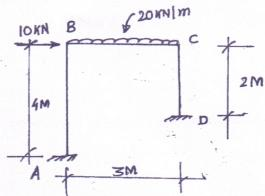
Q. No. 6 a) Analysis the pin jointed plane frame shown in figure and calculate the forces in all members. Take AE constant.
