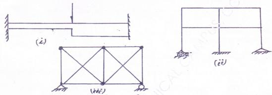
Q. No. 1 (b) Determine the horizontal displacement of joint 0 of the rigid jointed plane frame as shown in figure, due to change of temperature of member surfaces. Consider depth of all the members as 500mm. Take  $\alpha_{t=}$  12 X 10<sup>-6</sup> / O (10)
