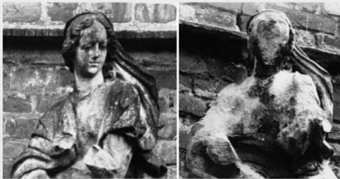
Effect of Acid Rain on Stone
