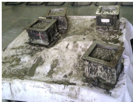
Fig 3.3: Table Vibrator Compaction
