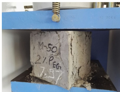
Fig 3.5: Failure of Cube
