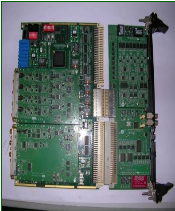
Figure 7: VME64X module with mezzanine cards
