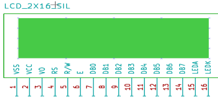
Fig12: PIN DIAGRAM OF LCD
