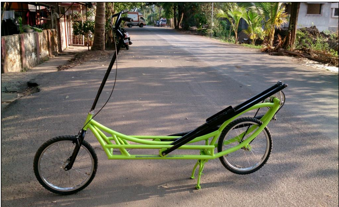
Fig 9.6.4:- Final look of ElliptiMove after completion of fabrication phase-II
