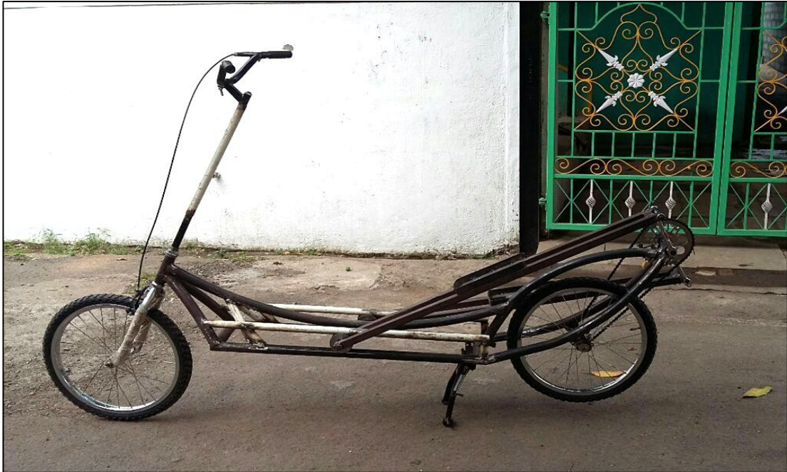
Fig 9.6.3:- Fabrication phase-II partially completed.
