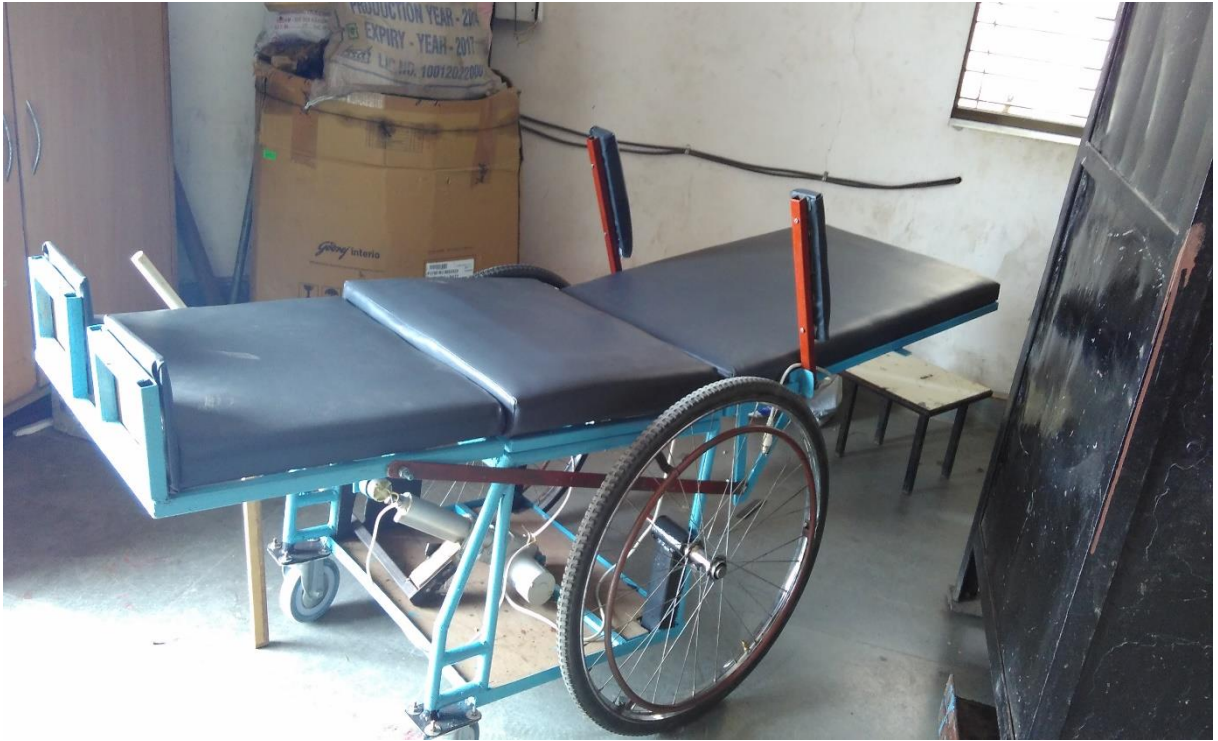
Fig 10.1. : Assembly of wheelchair with all three positions
