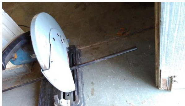
Fig. 6.1. Pipe cutting on cutter machine
