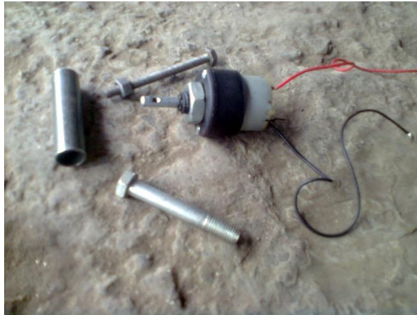
Fig. 7.3. Components of collinear actuators
