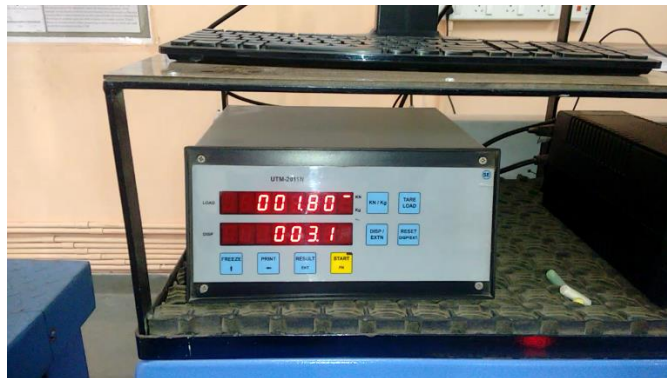
Fig. 7.12 Digital indicator showing applied force
