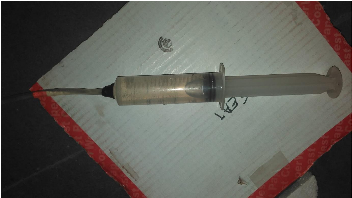
Fig. 3.2 Syringe used as actuator
