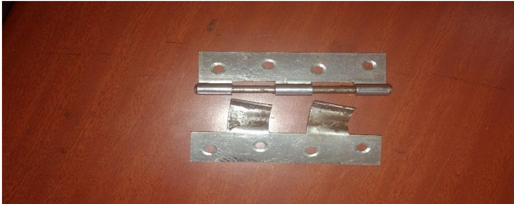
Fig. 7.15. Failure of hinges
