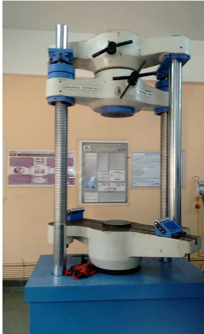
Fig. 7.13. Universal testing machine (UTM)
