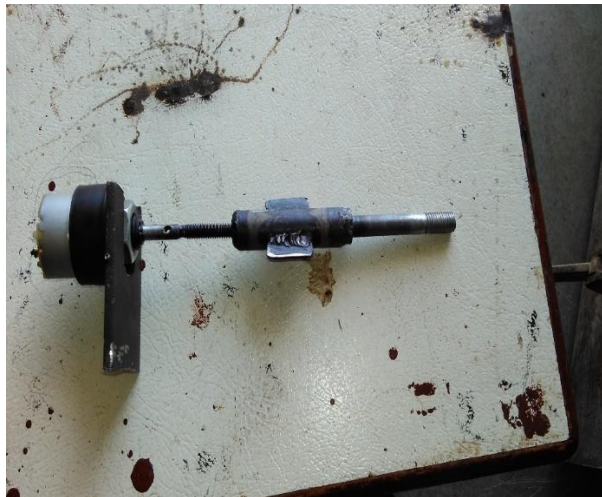
Fig. 7.4. Assembly of collinear actuators
