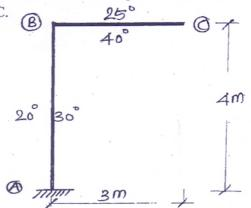
(b) Develop the stiffness matrix for prismatic member AB with reference to the 06 co-ordinates as shown in fig.
