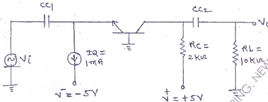
5. (a) For the Amplifier shown determine (i) Q point (ii)  $A_v$ ,  $Z_i$ ,  $Z_o$  10
