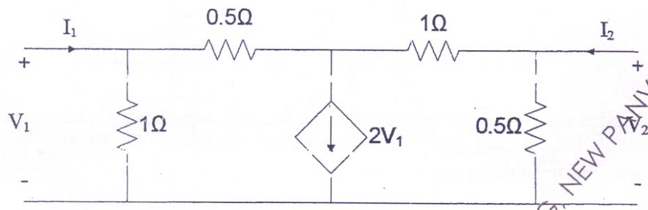
Q6 b) Calculate mesh currents in given circuit 10
