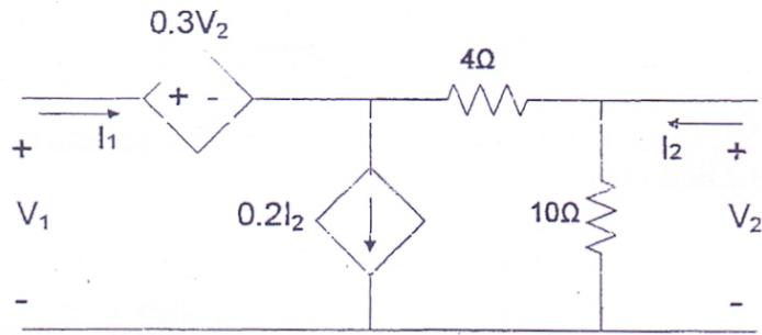
Q4 b) Determine the driving point impedance  $\frac{V_1}{I_1}$ , transfer impedance  $\frac{V_2}{I_1}$  and voltage transfer ratio  $\frac{V_2}{V_1}$  in the given network.
