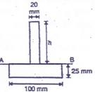
b) Find all support reaction. B is an internal hinge.
