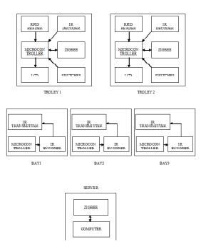
These units are integrated into a smart enclosed system and are tested to satisfy the functionality. The smart shopping cart will help shorten the checkout lines thereby helping the customers at retail stores. The customers will be able to scan the items themselves and the LCD screen on the shopping cart will keep updating the total. This will turn out to be very beneficial for the retail stores as more people will enjoy the shopping experience and come more often to shop.
