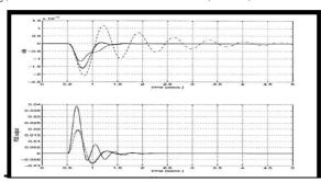
System response to 5% step disturbance at the voltage reference input of the AVR ----- no controller , ....... conventional , \_\_\_\_\_ QFT based . for different values of P Q and Xe.for wide range.
