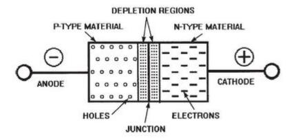
As holes enter the N region, they find number of donor atoms. The holes recombine with donor atoms. As donor atoms accept additional holes, they become positively charged immobile ions. Atoms on P side are acceptor atoms. The electrons diffusing from N side to P side recombine with the acceptor atoms on P side. As acceptor atoms accept additional electrons, they become negatively charged immobile ions. Such a large number of negatively charged ions get formed near the junction on P side.
