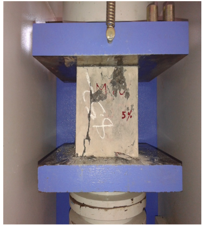
Fig. 5.1. Specimen in CTM after crushed
