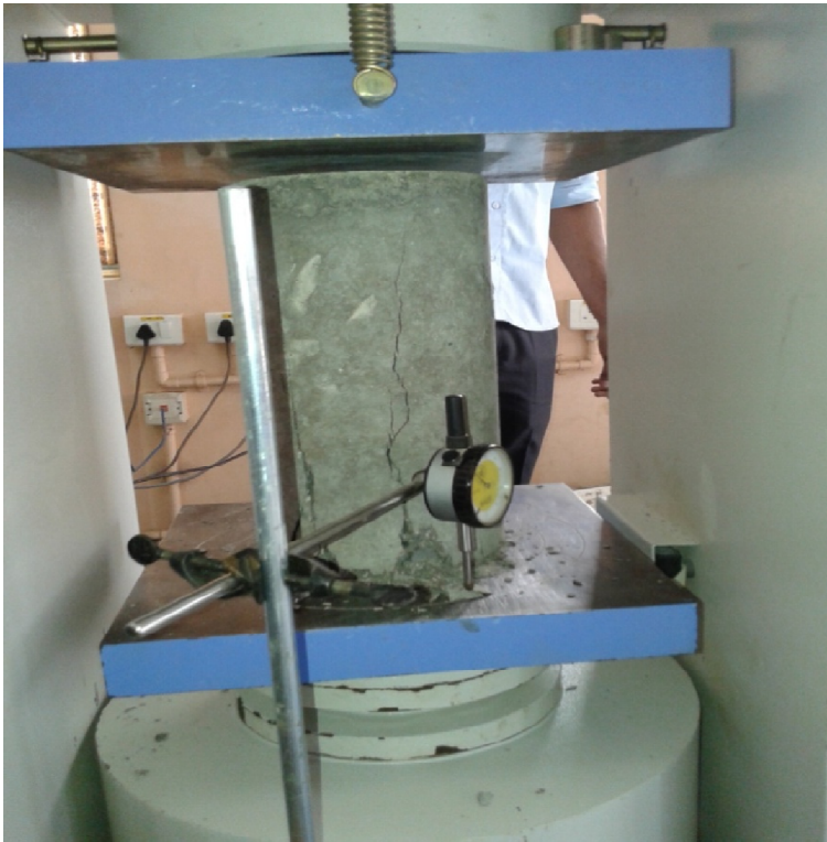
Fig. 5.1. Specimen in CTM after crushed
