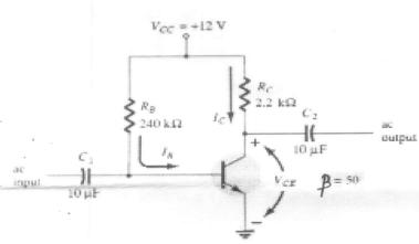
$V_{CC} = 12V$   $R_B = 240k\Omega$   $R_C = 2.2k\Omega$  B = 50  $C_1 = C_2 = 10MF$
