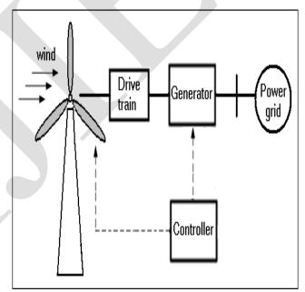
Fig.1 simple block diagram of wind turbine
