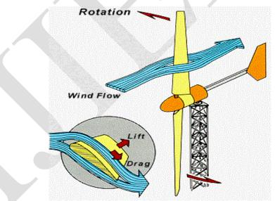
Fig.2 Principle of wind turbine aerodynamic lift [4]
