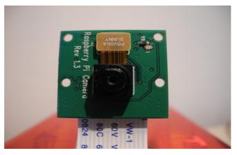
The camera consists of a small (25mm by 20mm by 9mm) circuit board, which connects to the Raspberry Pi's Camera Serial Interface (CSI) bus connector via a flexible ribbon cable. Installation involves connecting the ribbon cable to the CSI connector on the Raspberry Pi board. This can be a little tricky; otherwise you can damage the camera.
