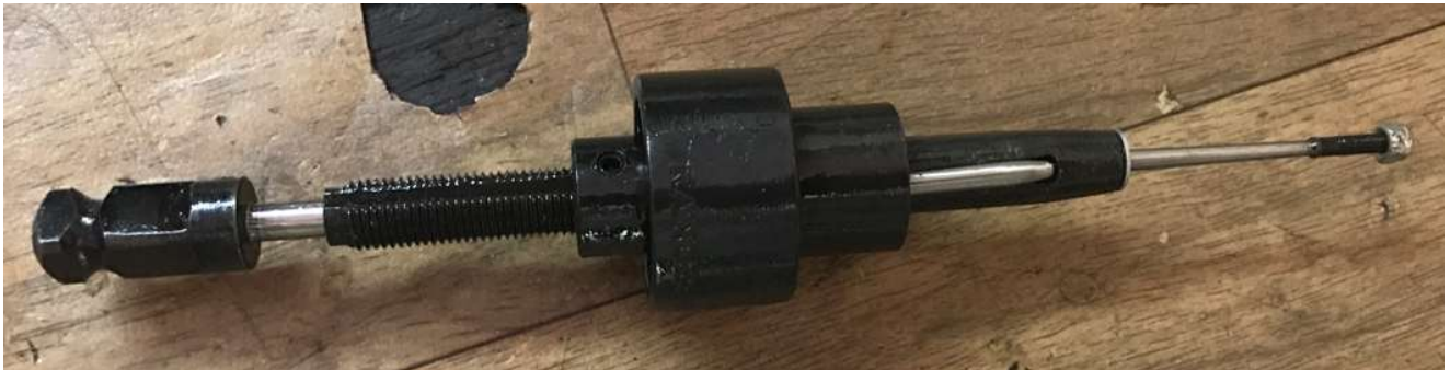
Fig. Tube Expander 805S
