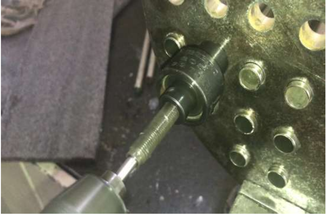
Fig. Expansion Process
