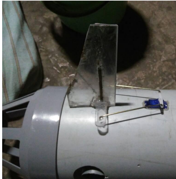
Fig 5.5 rudder and its mechanism
