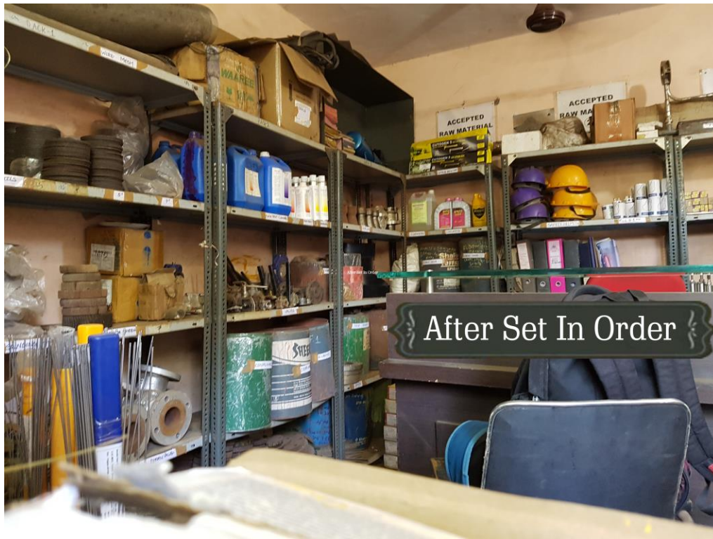
Fig 4.6: Overall presentation of store after implementing 5S: wherein all the inventories are sorted, kept in its place, cleaned and the disciplinary norms are maintained
