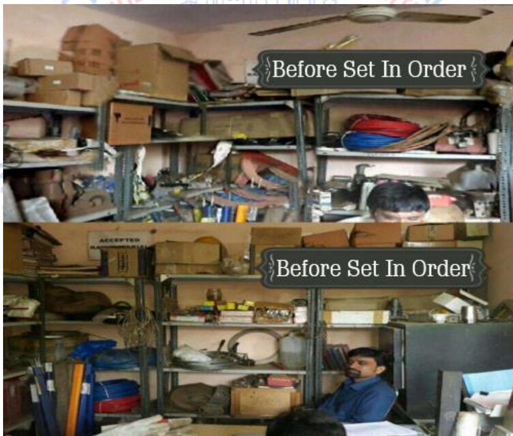
Fig 4.5: The overall presentation of the store before 5S: wherein all the inventories were not sorted in its place which made it difficult for the workers to hunt for the required tools
