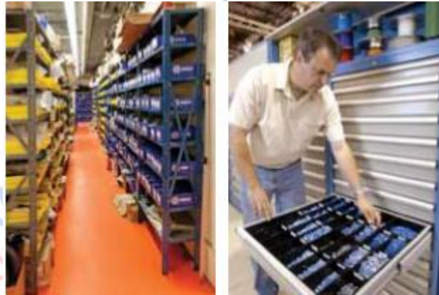
Fig 3.1: Open shelving (left) is very inefficient at storing small items. High density drawer and shelf storage (right) enables storage of small items in right-sized compartments, increasing cubic capacity and organization.
