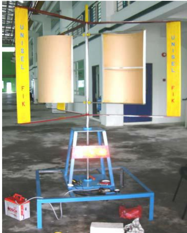
Fig.2.1 Illustration of the vertical axis wind turbine used to measure the power generation [14]
