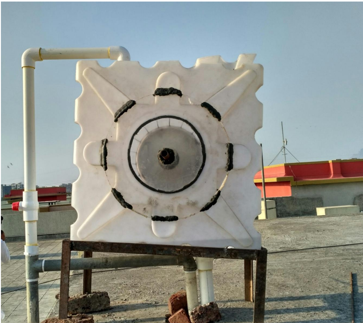
Fig.5.18 Actual set of Hydro Turbine
