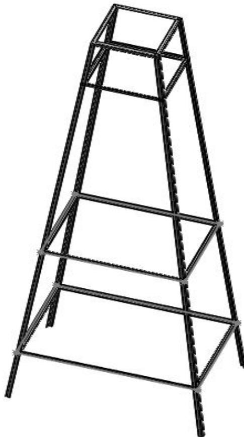
Fig.4.14 M.S angle tower
