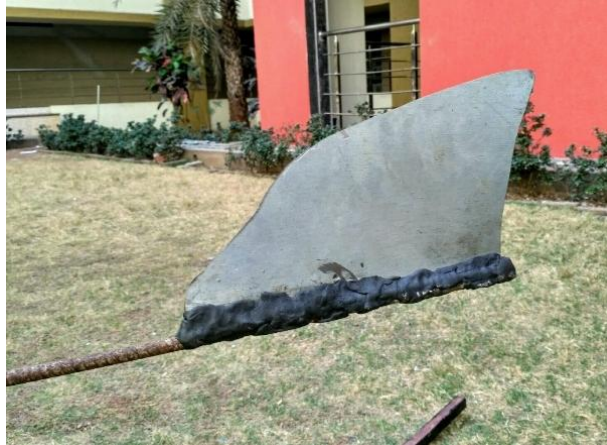
Fig.4.7 Tin sheet deflector
