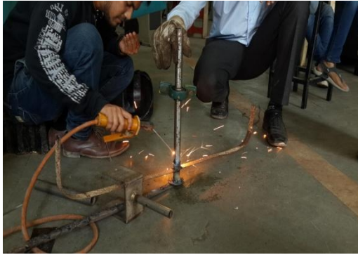
Fig.5.11 Welding of chassis
