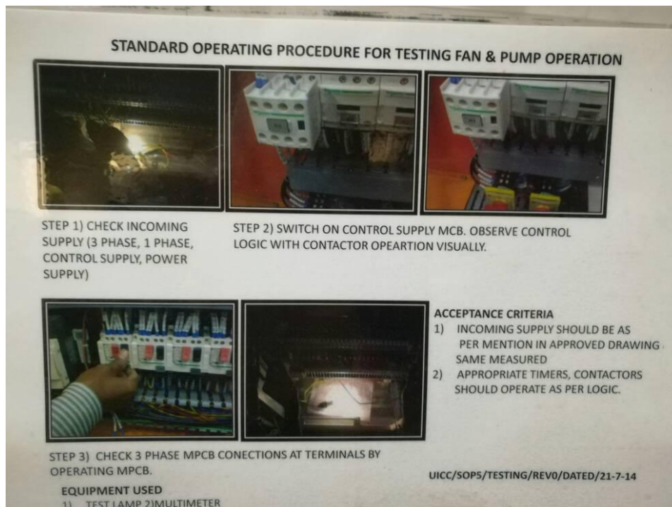
Fig. 6.16 Testing Fan & Pump Operation
