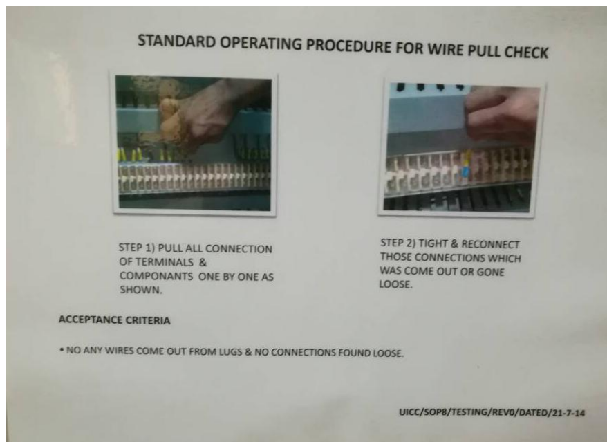
Fig. 6.12 Wire Pull Check
