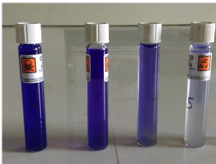
Figure 4.27 Effect of Inter electrode distance with time on colour removal
