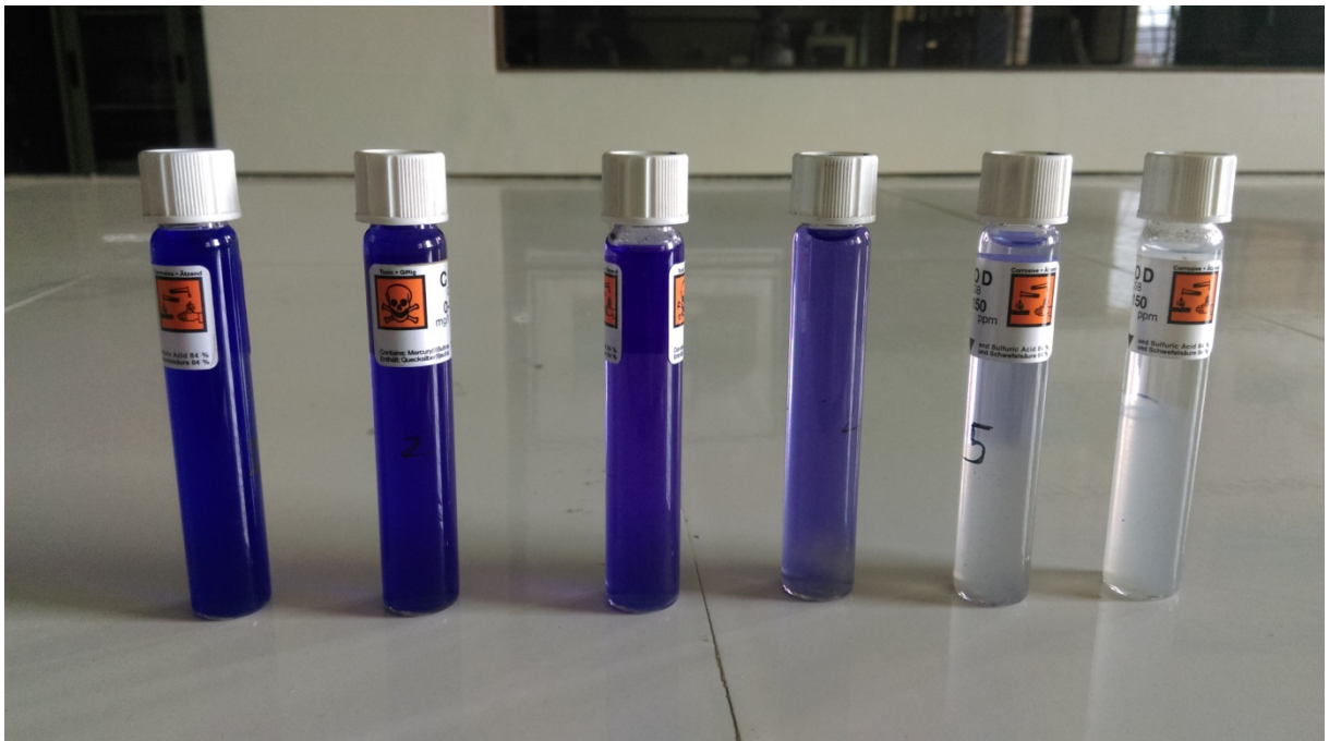
Figure 4.24 Effect of electrolyte dose with time on colour removal
