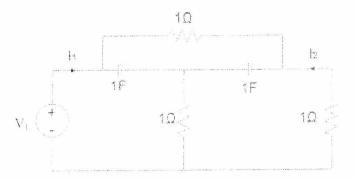
5. (a) A network and pole zero diagram for a driving point impedance Z(s) 10 are shown in figures. Calculate the values of the parameters R, L, G and C if Z(j0)=1.
