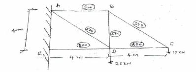
Q.5 (b) Draw ILD for members 4,5 and 6 of truss shown in fig. Assume that the load (10)
