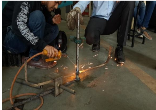
Fig.5.11 Welding of chassis
