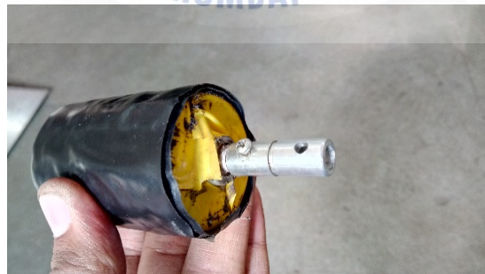
PICTURE :- COUPLING MOUNTED ON MOTOR SHAFT
