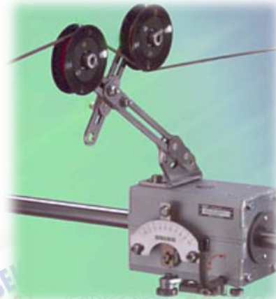
Fig. 2 Wire guide mounted on top of traversing nut.
