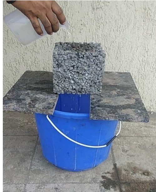
Fig 12 (b): Permeability test on 10 mm agg. concrete block
