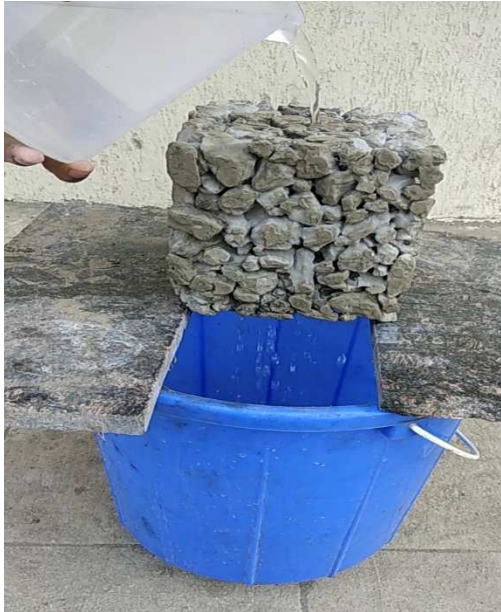
Fig 12 (a): Permeability test on 20 mm agg. concrete block
