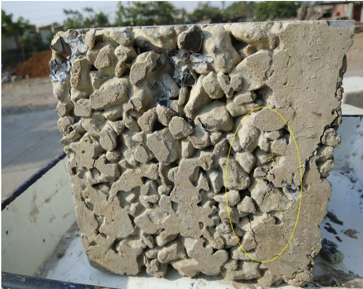
Fig 17: Concrete block after compression test
