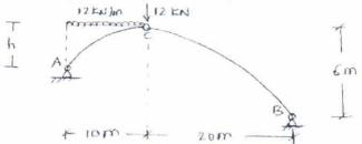
Q.3 (a) A pin jointed truss is loaded and supported as shown in figure. Determine the horizontal deflection of joint 'C' using Unit Load Method.
