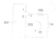
Q3 In the network shown, the switch is open for a long time and at t=0, it is closed. 10 Determine  $V_2(t)$ .
