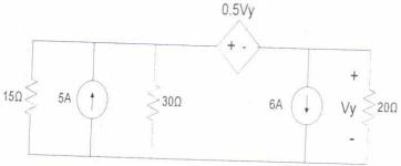
Q4 Find the Z parameters for the network shown. Hence find h 10 b) parameters.
