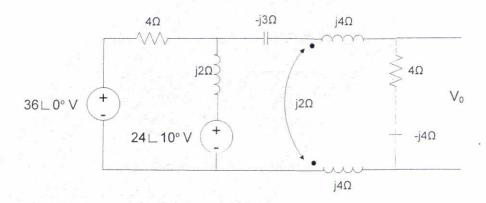
Q6 Find  $h_{12}$ ,  $Z_{12}$ ,  $Y_{12}$  and  $h_{22}$  for the given two port network.
