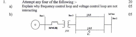
For the system shown if fault occurs at the middle of the line. Find transfer reactance between bus 1 and 2 by **NODE ELIMINATION** technique only
