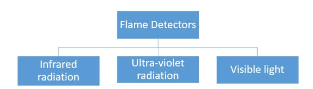
Apart from producing hot .gases., fire releases radiant energy in the form of ) Infrared light, ultraviolet light and visible lights. Flame detectors are classified based upon their ability to detect these different types of lights coming from a fire. Hence flame detectors are classified three main categories.
