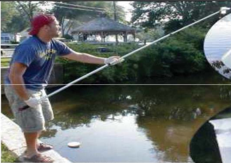
Poles are useful for sampling in basins (above) or in drains or wells (below.)
