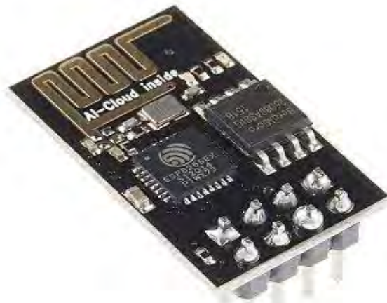
Figure 3.6: ESP WIFI module
