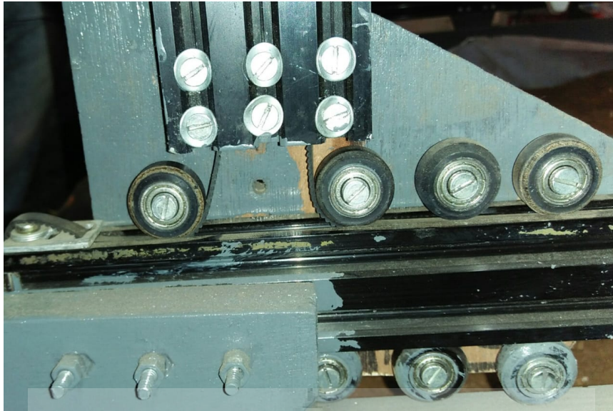
Figure 4.52: X-Axis Motion From Timing Belt to V-Wheels
