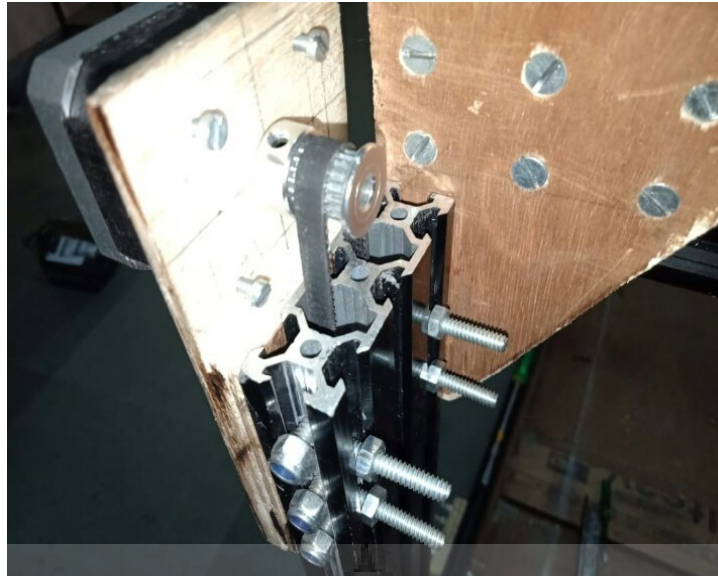
Figure 4.40: Mounting of brackets on top of column extrusion
