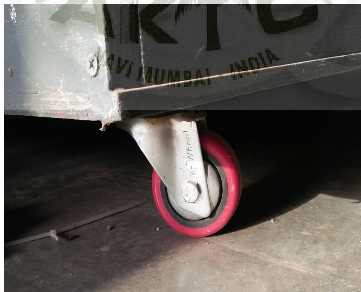
Figure 4.38: Mounting of Castor Wheels
