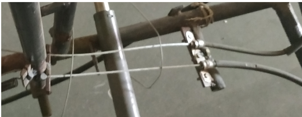
Figure 8.2: Attachment of brake cable to lever
