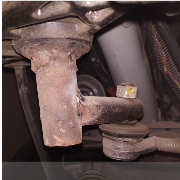
Figure 6.7: Ball joint attached to Aprilia Steering Column
