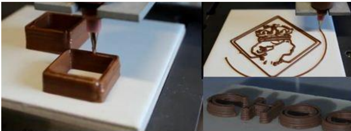
Figure 11 3D printing of chocolate [3]
