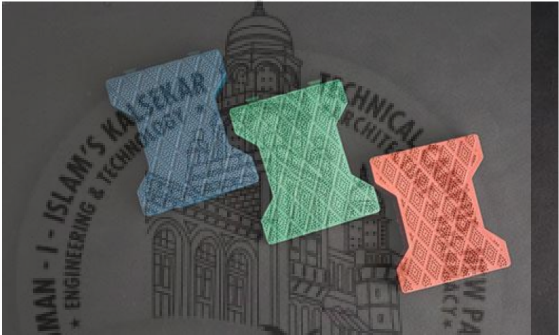
Fig 10: Recycled plastic paver blocks
