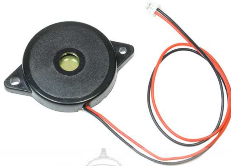
Figure 6.12 - Buzzer for Pixhawk PX4. [27]
