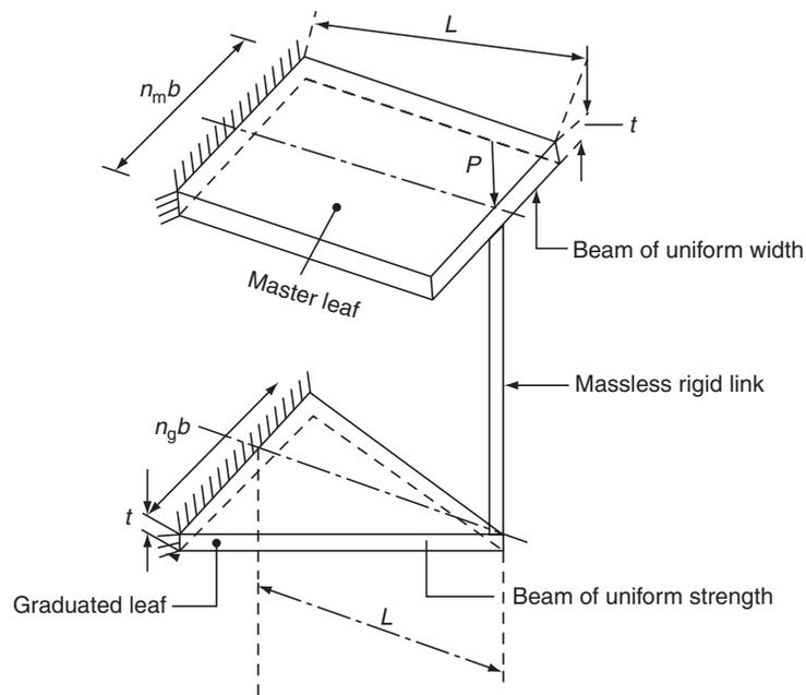
Figure 17.7 Parallel assembly of cantilever leaf springs.
