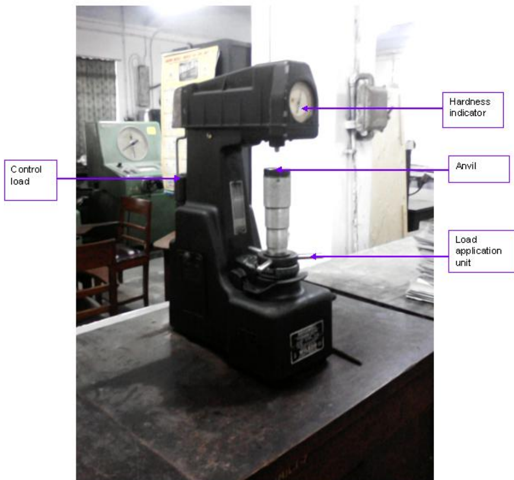
Figure 1 Rockwell hardness tester.
