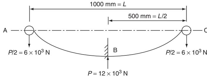
**Figure 17.8** Arrangement of beams in Example 17.2.
