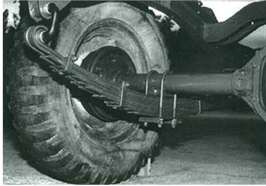
Figure 17.2 Leaf spring in an automobile.
