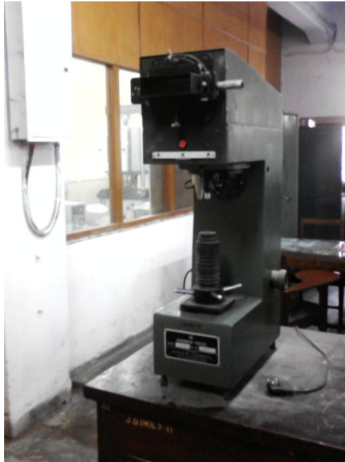
Figure 3 Vicker's hardness test.
