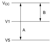
$A = V_{CC} - V_5$
