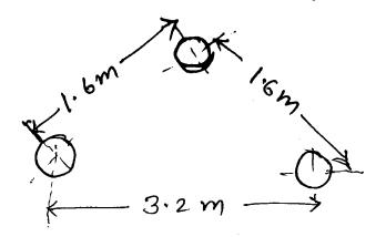
The conductor diameter is 0.8 cm.
