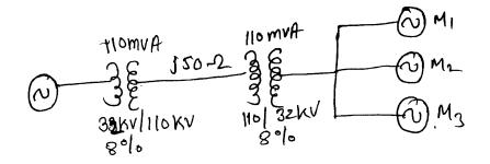
The motors have rated inputs of 30 mVA, 20 mVA and 50 mVA at 30 kV with 20% subtransient reactance. The generator ratings are as shown in diagram. Selecting generator rating as the base quantity in generator ckt. Draw P. U. reactance diagram.
